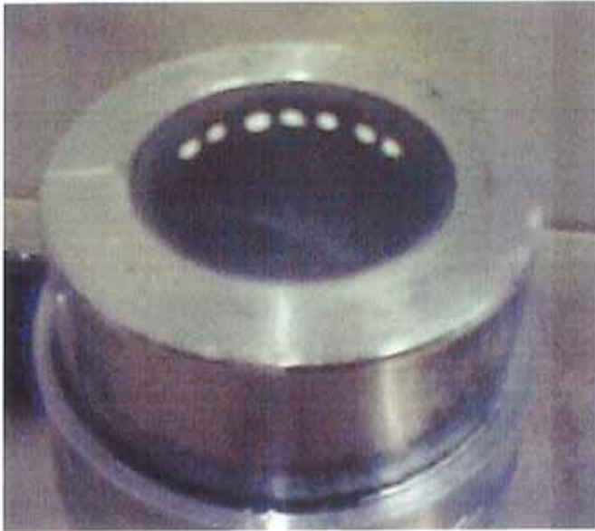
Figure 2. Specimen in rig clamp showing pattern for optical measurement.
