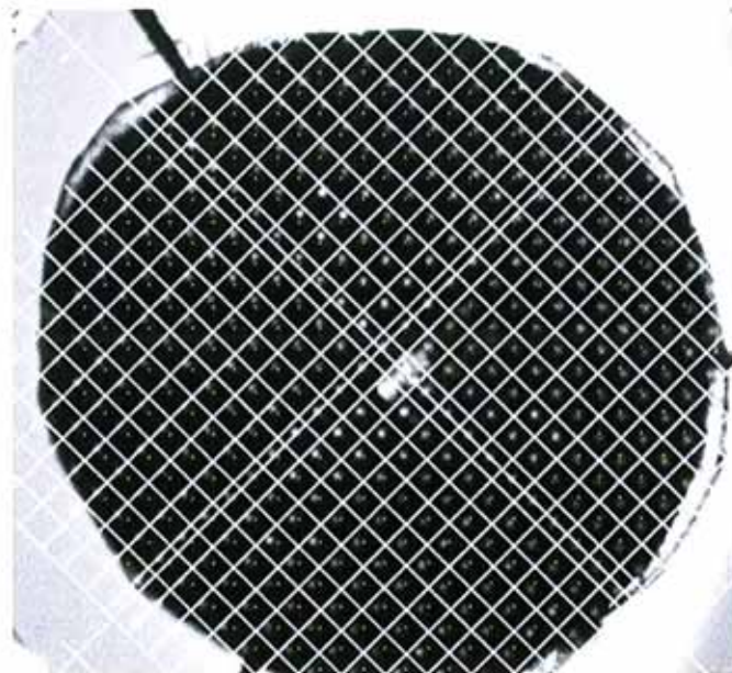
Figure 5.5 An example of the manual inspection image displayed after executing action 2. The subfield grid and reference HS spots are visibly misaligned indicating that the alignment process is not at an endpoint. This particular example also reveals a number of issues that the operator needs to address including infrared saturation of the alignment channel and a large unwanted central reflection in the sensing channel.
