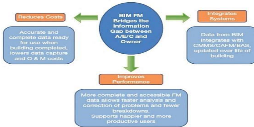
Fig 2.6: Main benefits that can be achieved from BIM FM integration - Source Teichloz (2013).
