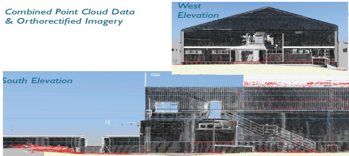
Fig 4E: Combined point cloud data and orthorectified imagery
