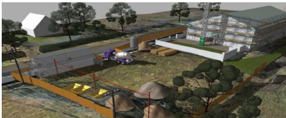
Fig 7.7: 4D design illustrating the logistics and site layout of the technology pilot 2013
