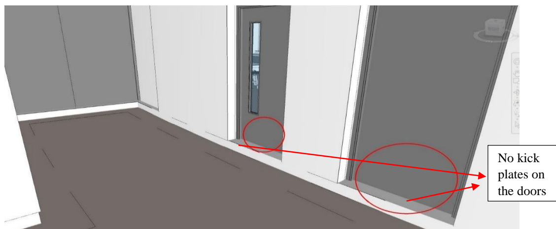
Fig 9.3: Illustration of door selection in the DoES School model with no kick plates
