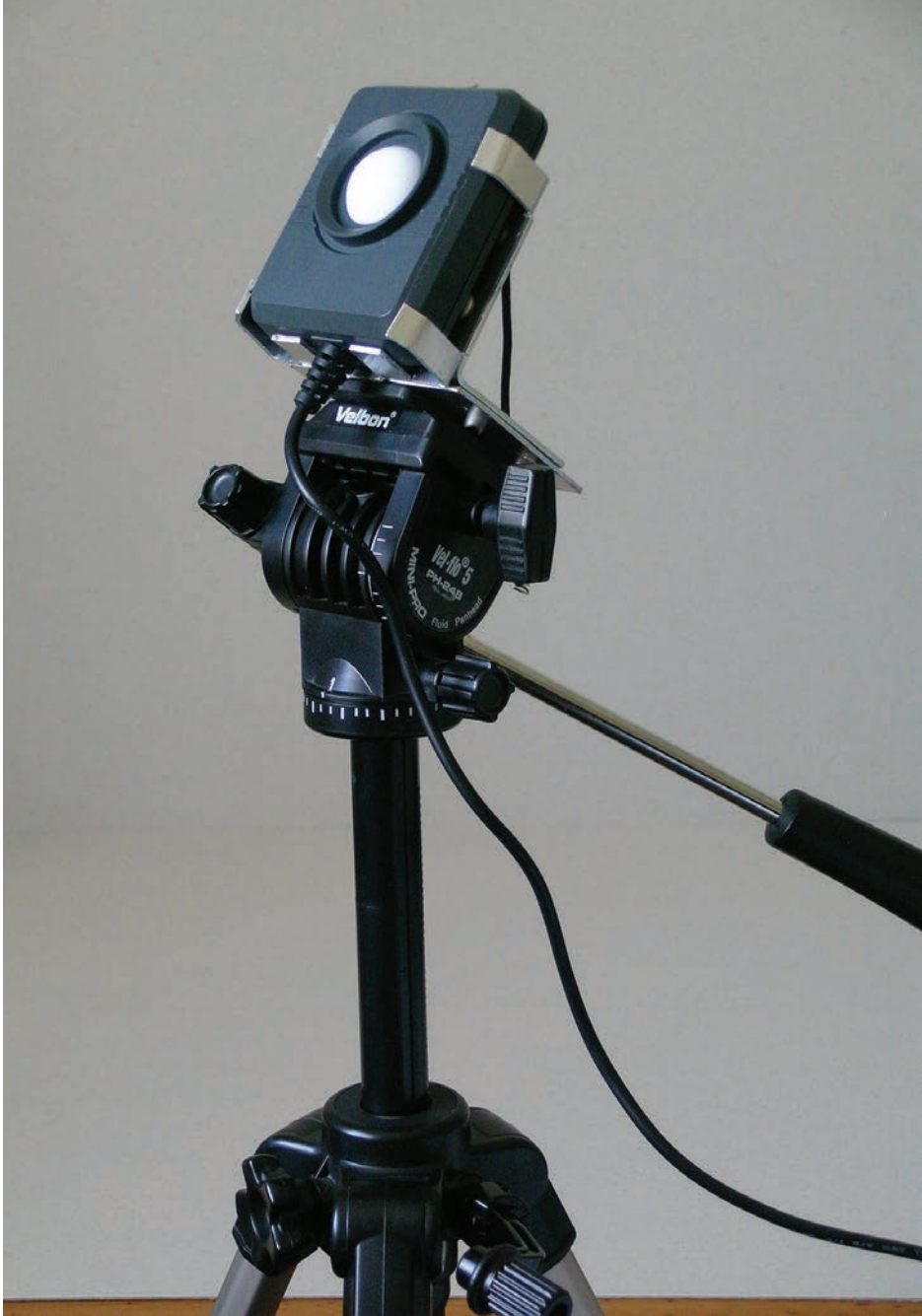
FIGURE 6.14 The photocell tilted to +35^\circ relative to the horizontal plane, and ready for measuring the three-dimensional illumination distribution.
