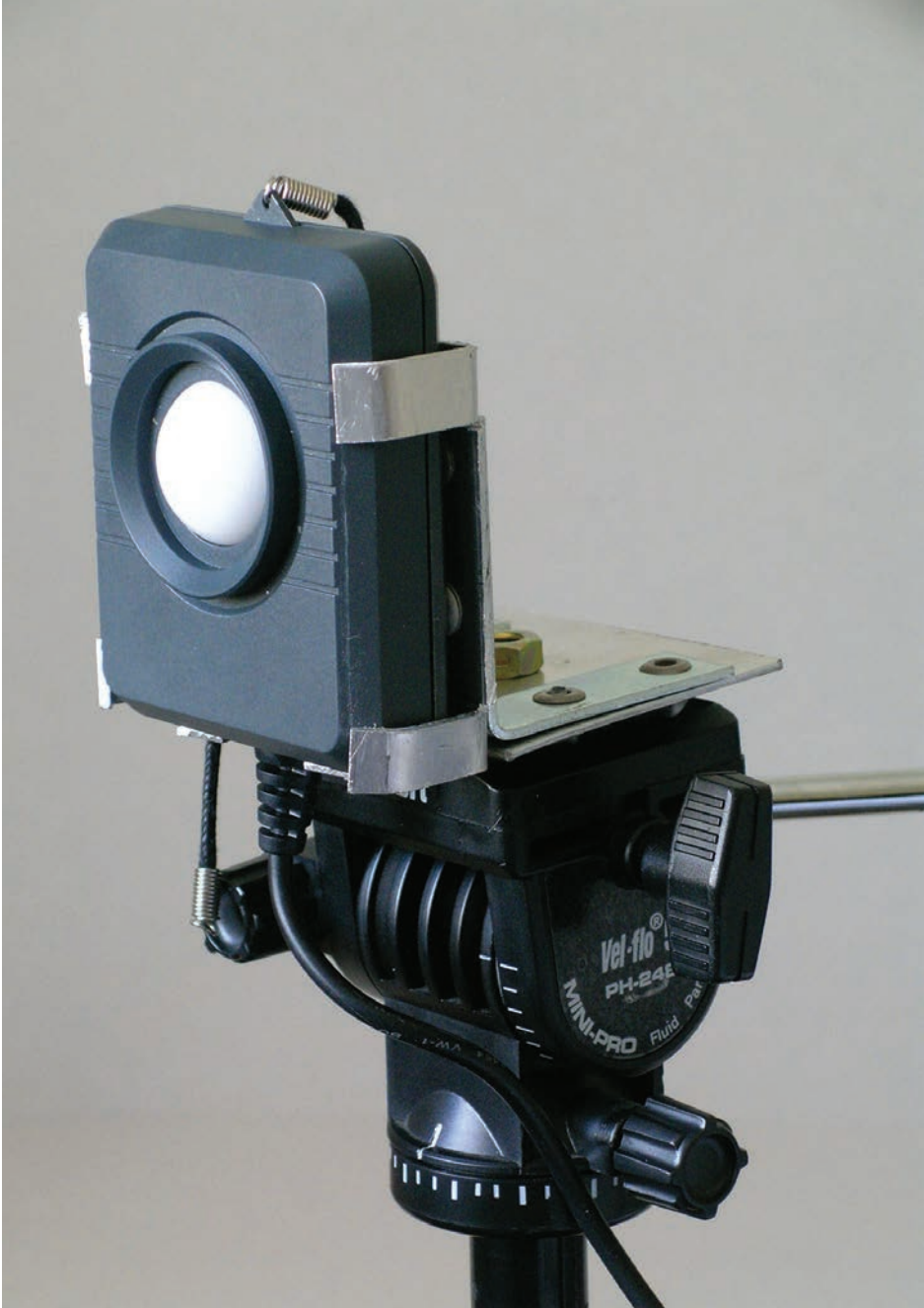
FIGURE 6.13 A photocell head mounted on a right-angle bracket, onto a photographic tripod.
