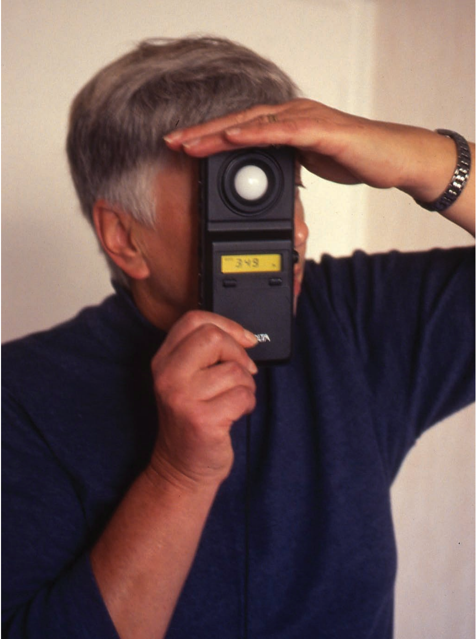
FIGURE 6.9 A simple way of making an approximate measurement of MRSE using a conventional light meter. Expose the meter to a wide view of the space avoiding, as far as possible, windows and other light sources, and shield direct light from any overhead luminaires.
