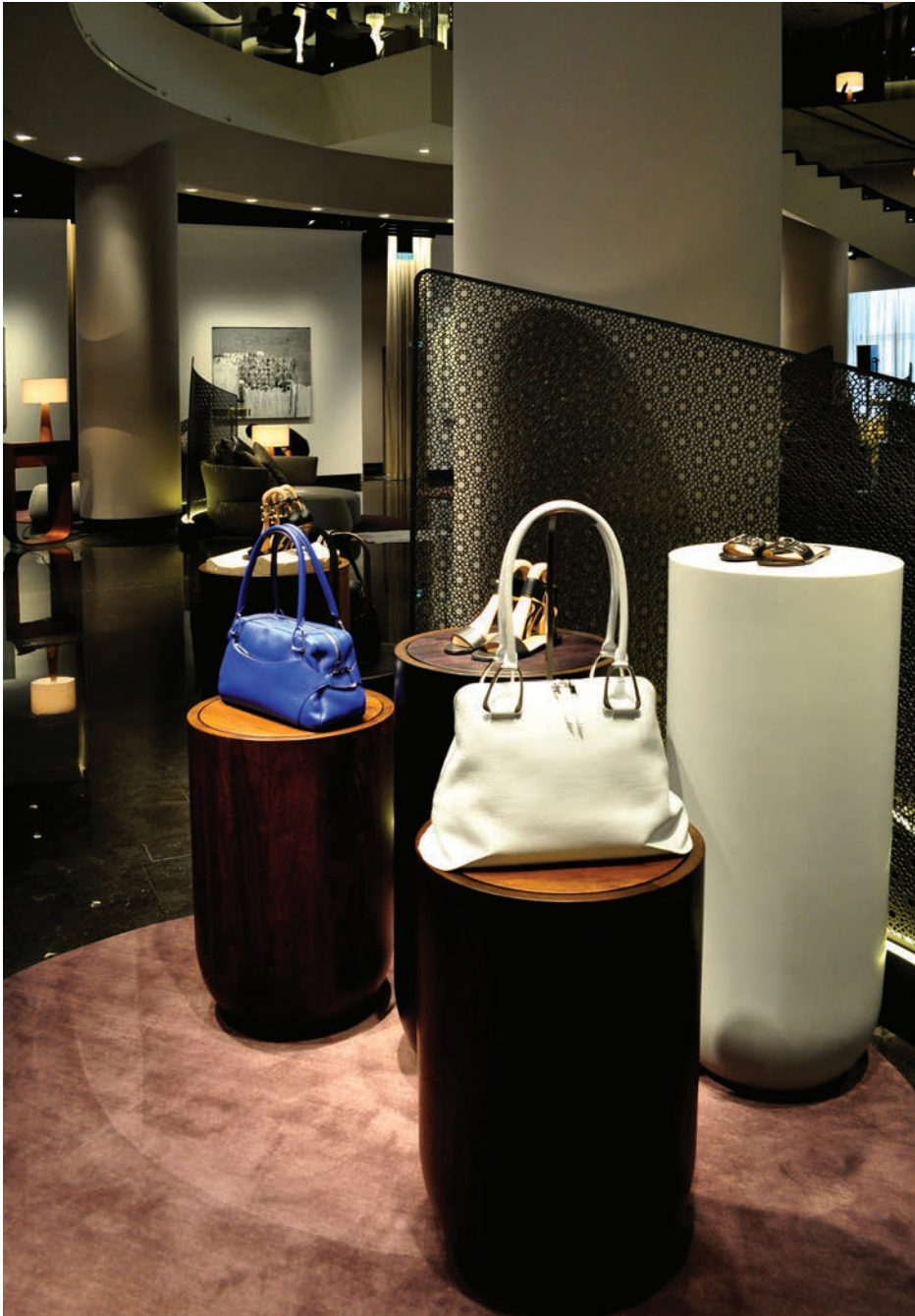
FIGURE 5.5 QELA – In this display area, which is adjacent to the central area, the lower mean room surface exitance (MRSE) level has the effect of strengthening the shading patterns. Interior design by UXUS Design, Amsterdam; Photography by Adrian Haddad; Lighting by dpa lighting design.
