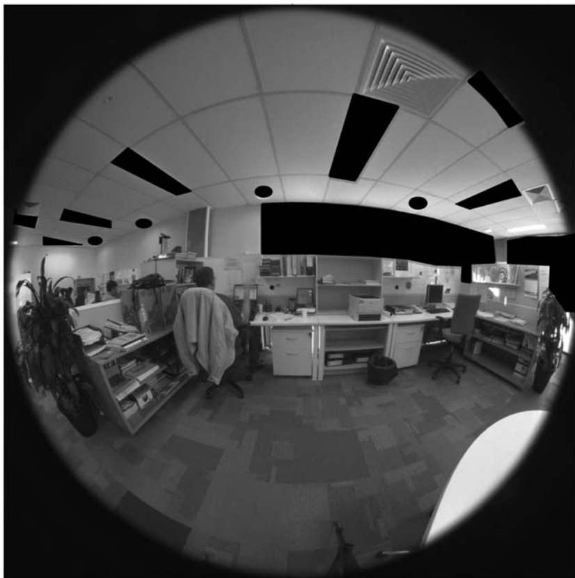
Figure 2. Full-field high dynamic range image (HDRi) for which each pixel is calibrated on a luminance-based scale. Light sources, both windows and luminaires, are shown blanked out as they will be disregarded for calculating mean room surface exitance (MRSE).
