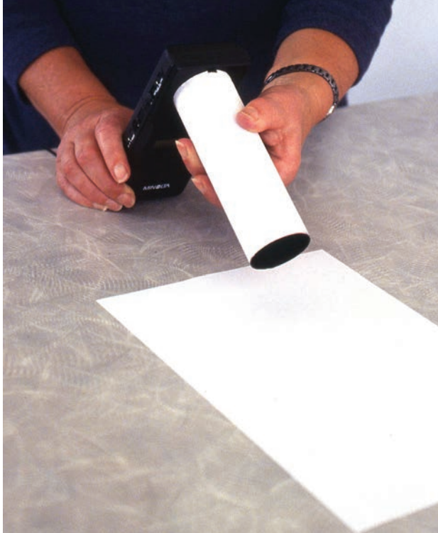
FIGURE 6.1 Measuring surface reflectance, using an internally blackened cardboard tube fitted over an illuminance meter. Comparative readings are taken of the surface, avoiding specular reflections, and of a sheet of white paper.
