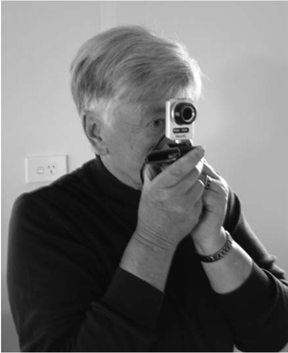
Figure 5 Using a 'measuring eye' (in this case a webcam) to capture an image of the field of view, including direct light from the luminaires
