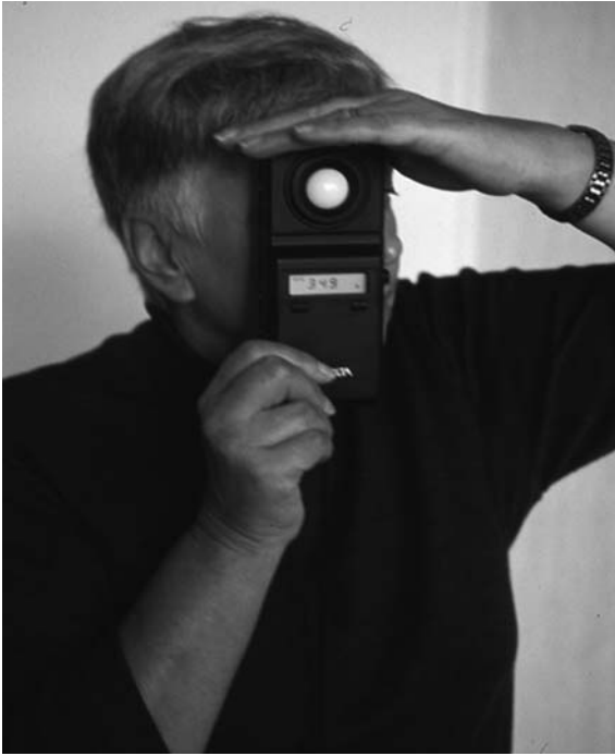
Figure 4 Using an illuminance meter to gain an indication of mean room surface exitance. Direct light from overhead luminaires is shielded, so the meter responds to reflected light from room surfaces arriving at the eye
