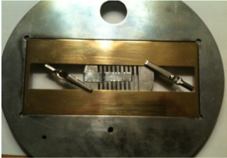
Figure 20. Bespoke mask used for evaporating Indium Oxide pattern in Edwards 306E system.
