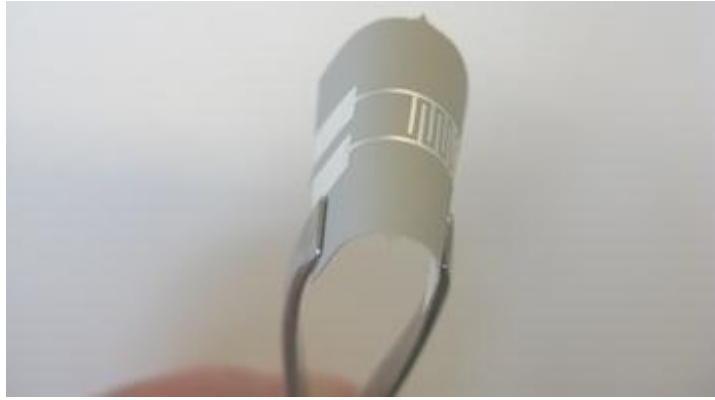
Figure 36. Optical image of the 3 pair IDE microwave sensor, which is bent to illustrate the flexibility of the polymer substrate [177].
