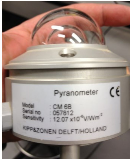
Figure 54. Pyranometer from Kipp & Zonen, for measuring the simulated solar irradiance/light intensity.
