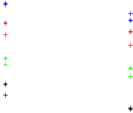
Figure 6.3 Examples of adjusted arrays at the Rx showing Y-dimension shifts only. The crosses mark the original position and star the final positions.
