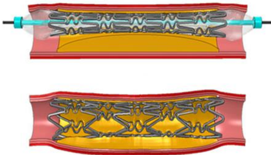
Figure 3.6: Deployment of the BX-Velocity stent within an idealised model of an atherosclerotic coronary artery using a realistic model of a balloon-tipped catheter, as described by Conway et al. [58].
