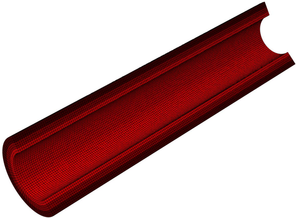
Figure A.21: Discretised CS model of the coronary artery containing 95,424 reduced-integration continuum elements (Mesh 3).
