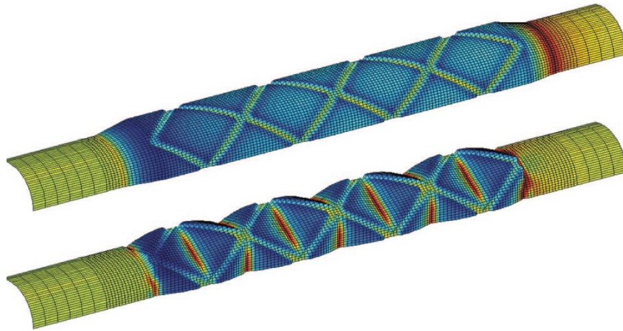
Figure 3.7: WSS distribution predicted upon the luminal surface of two stented coronary arteries that featured circular (top) and polygonal (bottom) cross-sections, as described by LaDisa et al. [78].
