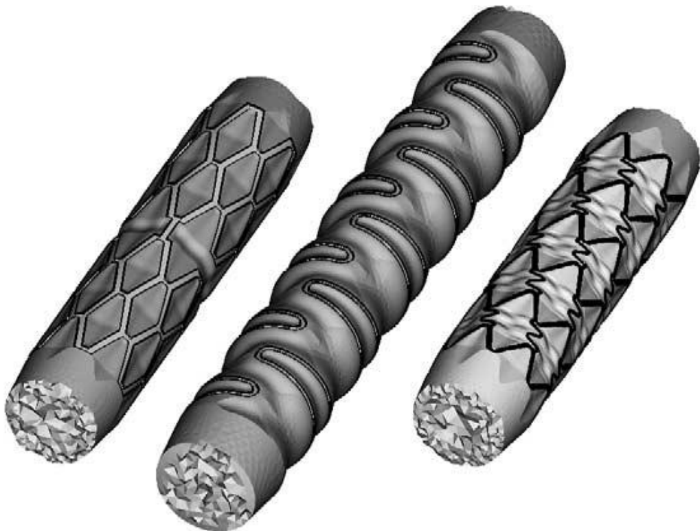
Figure 4.9: Solid models of the LAD arteries implanted with (from left to right) the PS stent, the GR-II stent and the Bx stent from Murphy and Boyle (2010). 172
