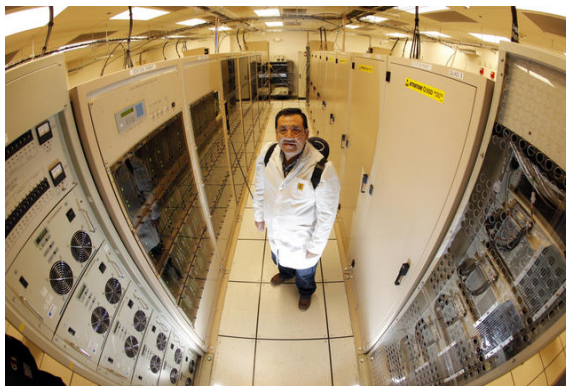
Figure 2.7: Technician breathing oxygen at the Alma Correlator, the world’s newest and highest high performance computing system with over 134 million processors [39].
