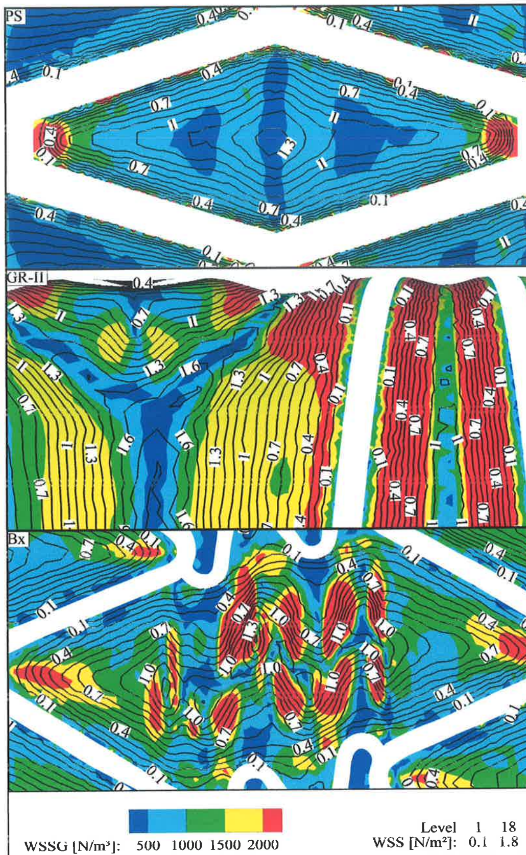
Figure 6-22: Contour plots of WSSG near the PS, GR-II and Bx stent struts with overlaid line contour plots of WSS (labelled by magnitude [N/m 2 ]).
