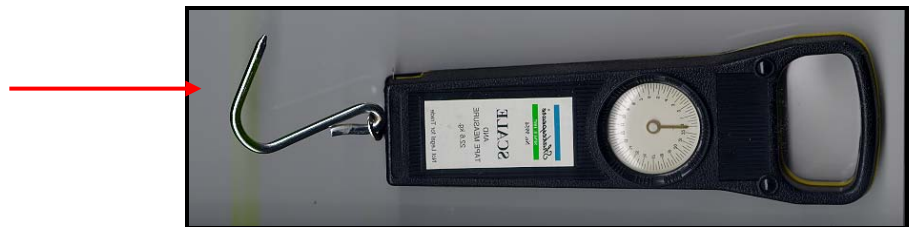
Figure 2.5 Scanned Image of Force Metre used to Measure Torque
