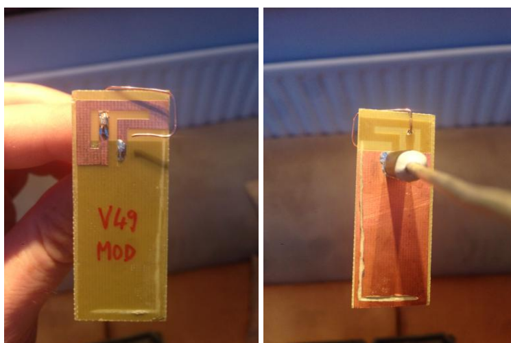
Figure 31: The empirical modifications made to the V49 prototype monopole side (left) and ground plane side (right).
