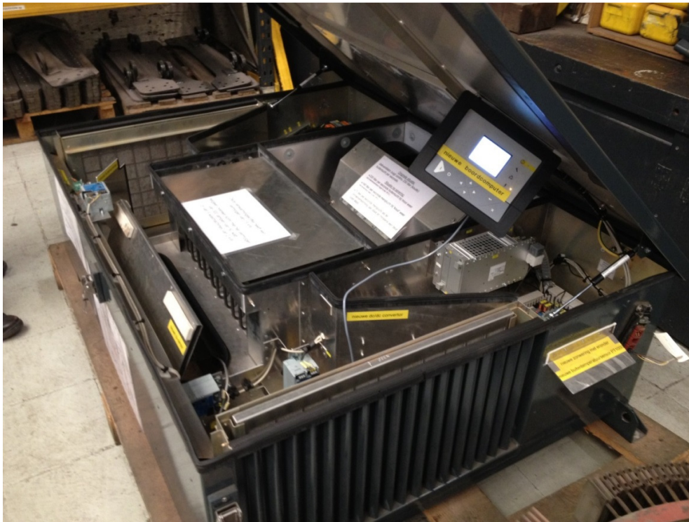
Figure 7: De lijn Modified Heating and Ventilation Unit [82]
