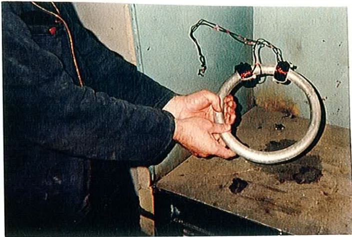
Figure 2.8a The aluminium ring flywheel with a single-phase induction-machine winding
