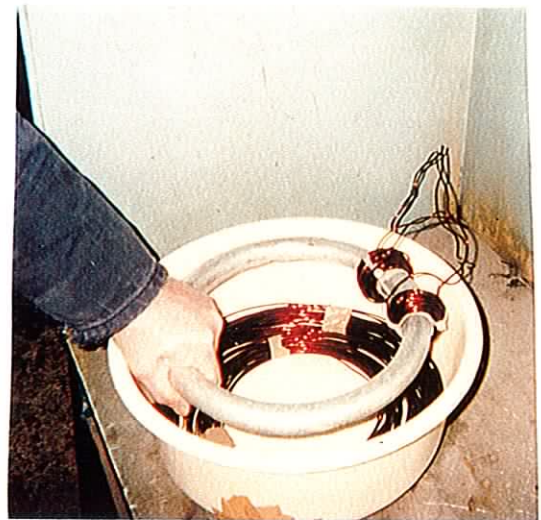
Figure 2.8b The ring flywheel in its levitating position over the uncovered basin containing the water-cooled ironless bearing windings
