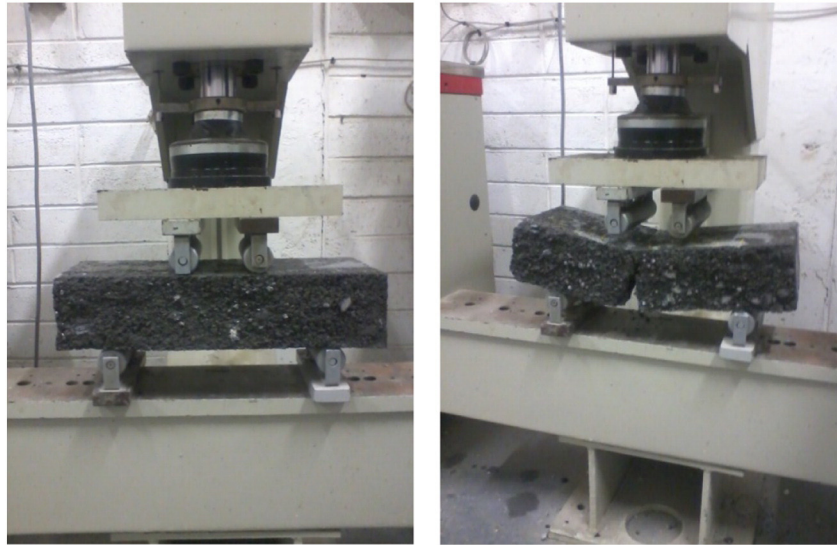
Fig. 3. Masonry block undergoing flexural loading.
