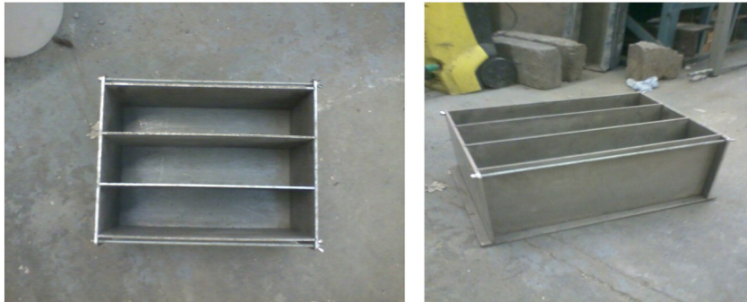
Fig. 1. Stainless steel moulds used to cast the masonry blocks.
