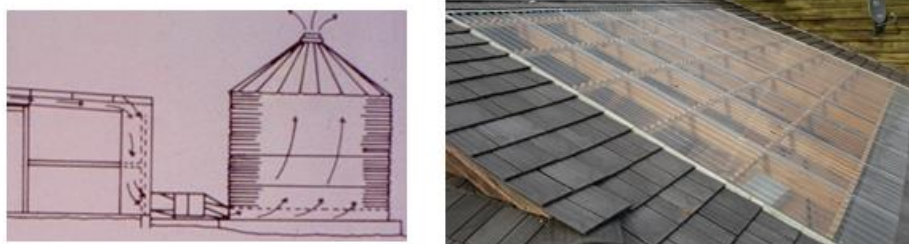
Figure 9. A roof-mounted air-heating solar collector and the integration of air-flow to a drying silo
