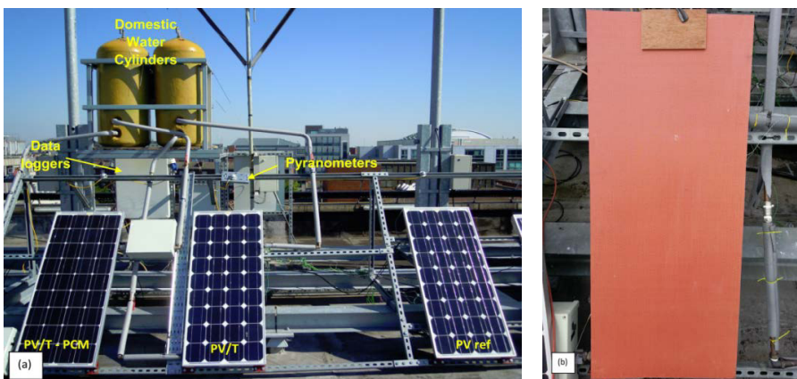
Fig. 2. (a) Experimental set-up (b) Heat mat
