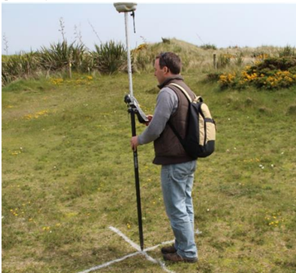
Figure 3. GCPs set on site for RPAS surveying.
