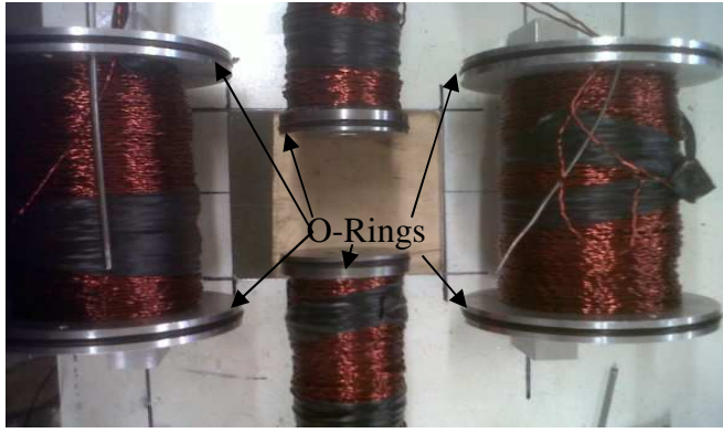
Figure 3a Coils wound with corrugated wire
