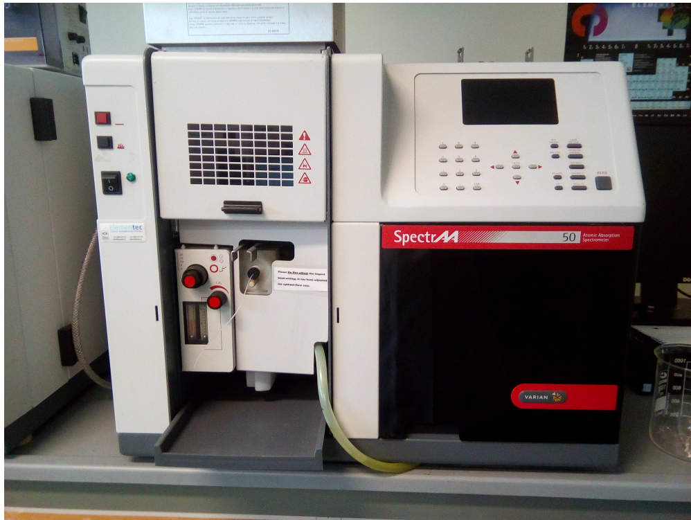
Figure 3.2: Varian 55B AA spectrometer (Varian Inc.) located in the facilities of TU Dublin.
