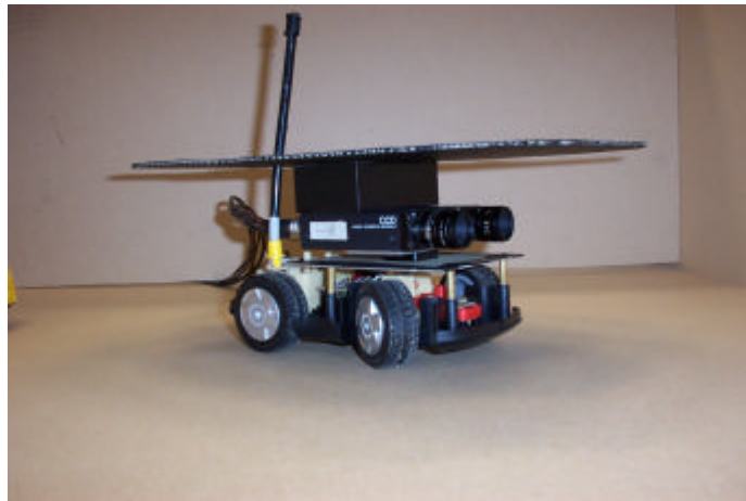
Figure 1 Mobile remote controlled stereo vision unit
