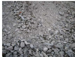
Figure 4.5 Undersize recycled concrete
