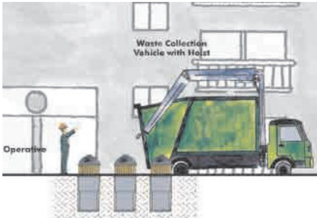
Figure 6.7: Deep Storage Waste Collection Vehicle
