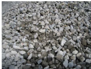
Figure 4.4 Oversize recycled concrete
