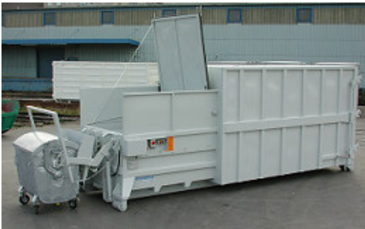
Figure 6.3: Waste Compactor and Container
