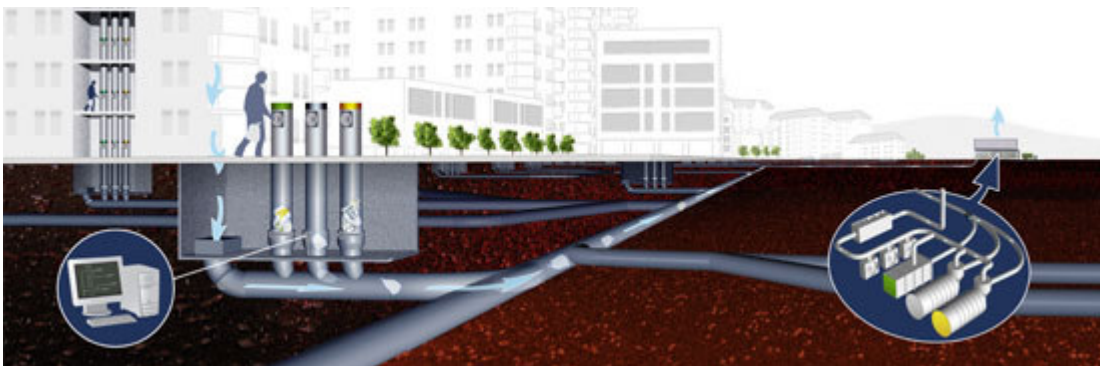
Figure 6.8: Schematic of Envac System
