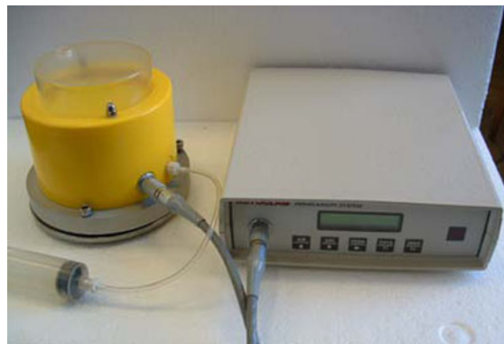
Fig. 4 Autoclam permeability apparatus [14]
