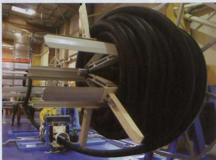
Uponor's new decoiling machine reduces and simplifies the process of straightening, cutting and recoiling pipes.
