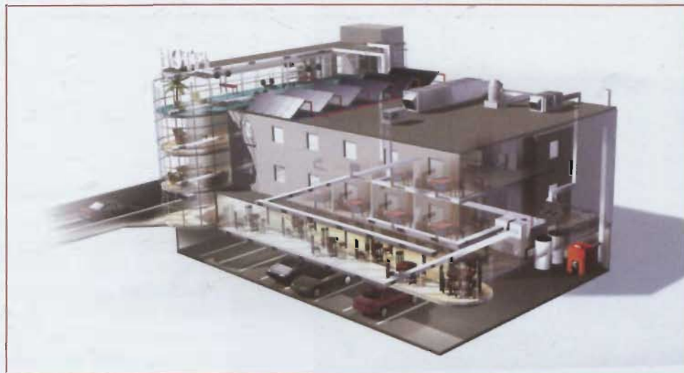
Schematic showing a hotel installation of the new Wolf KP Top air handling unit
