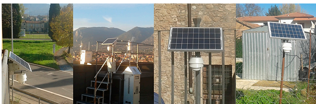
Figure 2. Smart samplers (SMART SAMPLER Fai Instruments, Fonte Nuova, Roma (RM), Italy) installed in 4 of the 23 monitoring sites of Terni.
