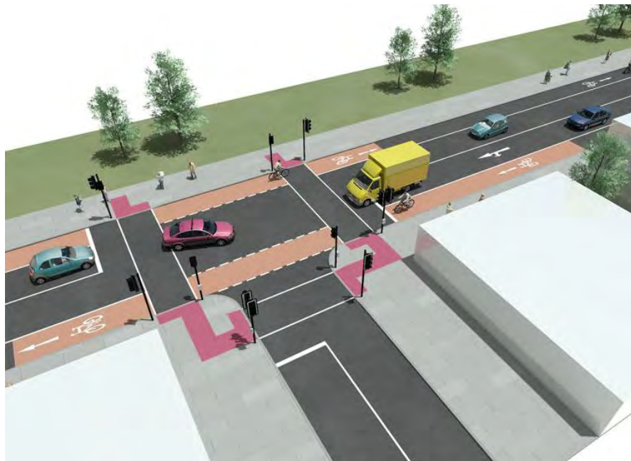
Figure 1.0: The National Cycle Manual' Cross roads planning detail (NTA, 2012).
