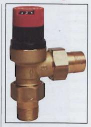
mechanism that prevents flow through the bypass while system valves are open, and increases water flow automatically as valves close. This raises energy efficiency by minimising bypass flow while, at the same time, providing a safe flow path around the boiler as specified in Good Practice 302.
