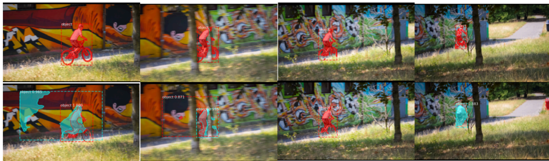
Figure 4.12 Ground-truth vs predicted segmentations for bmx-tree video sequence. The top row shows frames from the sequence at an interval of 20, superimposed with the ground-truth and the bottom row shows the same frames superimposed with the predicted segmentations.
