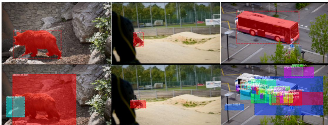
Figure 4.2 Some sample segmentations before training on the DAVIS dataset — the top row shows the images superimposed with the respective ground truths, the bottom row shows the images superimposed with the predicted segmentations of identified objects by the model with only the pre-trained backbone weights.
