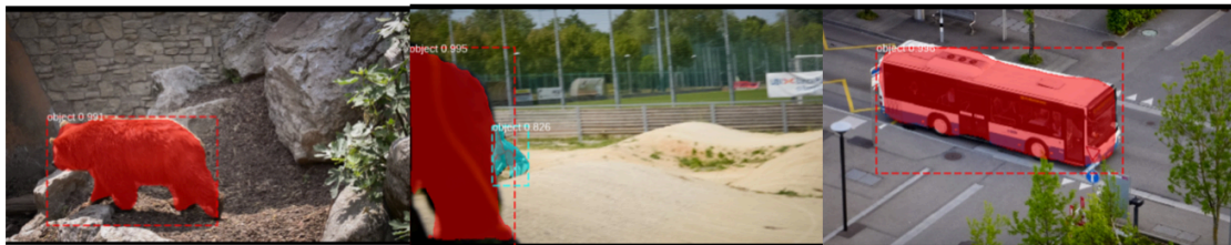
Figure 4.3 Segmentations for the same images after one additional epoch of training the head of the network architecture on the DAVIS dataset.
