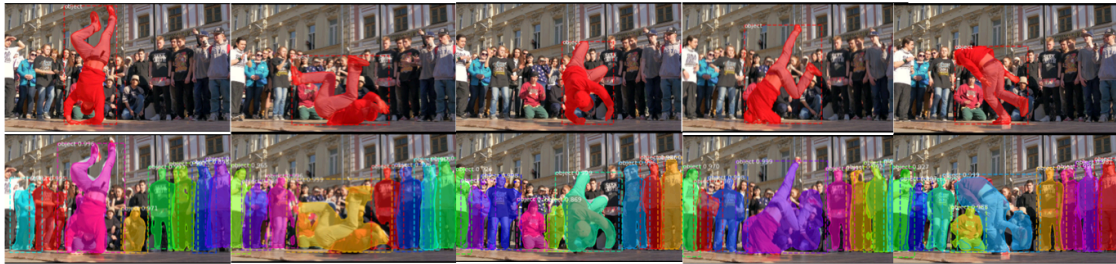
Figure 4.14 Ground-truth vs predicted segmentations for breakdance video sequence. The top row shows frames from the sequence at an interval of 20, superimposed with the ground-truth and the bottom row shows the same frames superimposed with the predicted segmentations.
