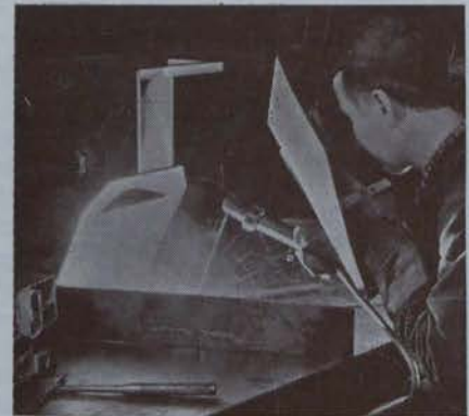
A Bahco workshop fan being used to extract welding fumes. The collecting hood is one of the Standard range of accessories.
