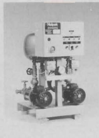
• The compact Holpak HCH booster pump set series for domestic light commercial applications: Duty 2 m 3 /Hr at 30 m head.
