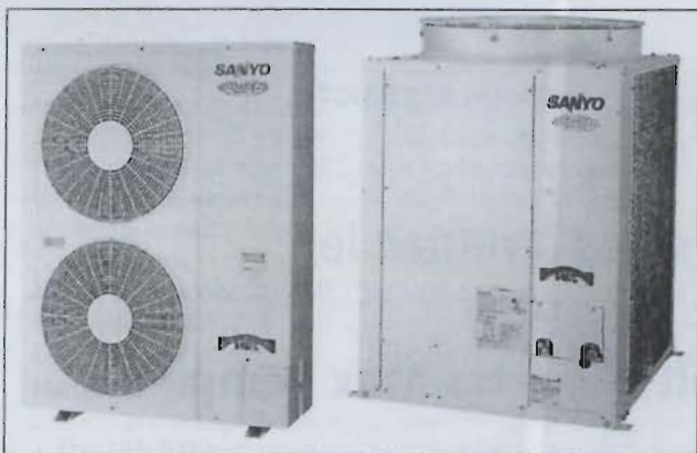
Sanyo Super ECO Multi Series – Instead of an inverter, the Super ECO MULTI system uses a super power control compressor and an external save valve to control capacity. This results in reduced harmonic wave emissions. Details from Redbro.
