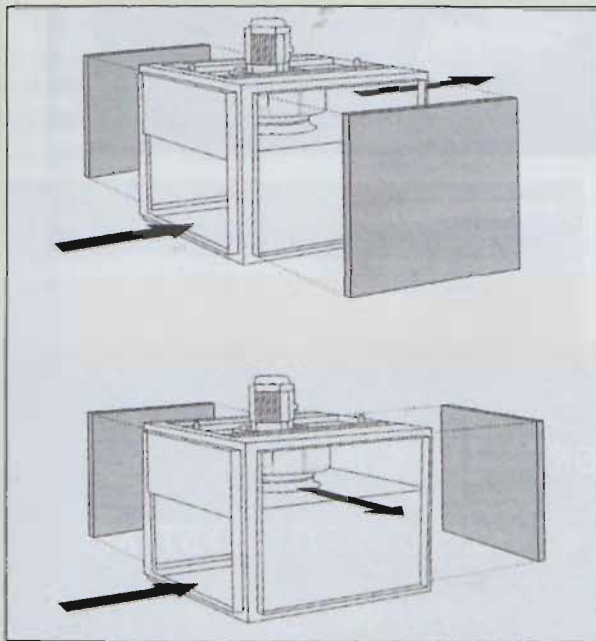
Installation options — The ILHT series of centrifugal in-line fans offers a truly flexible solution to installation whereby the configuration of both the inlet and discharge ports can be changed by simply altering the positioning of casing side panels.
