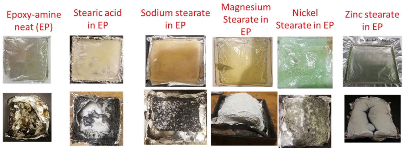
Figure 6.29 Unburnt (top) and burnt (bottom) pictures of epoxy-amine composites of different stearate salts.
