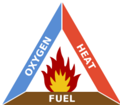
Figure 1.8 Fire triangle emphasizing the importance of three components required for a sustainable fire.
