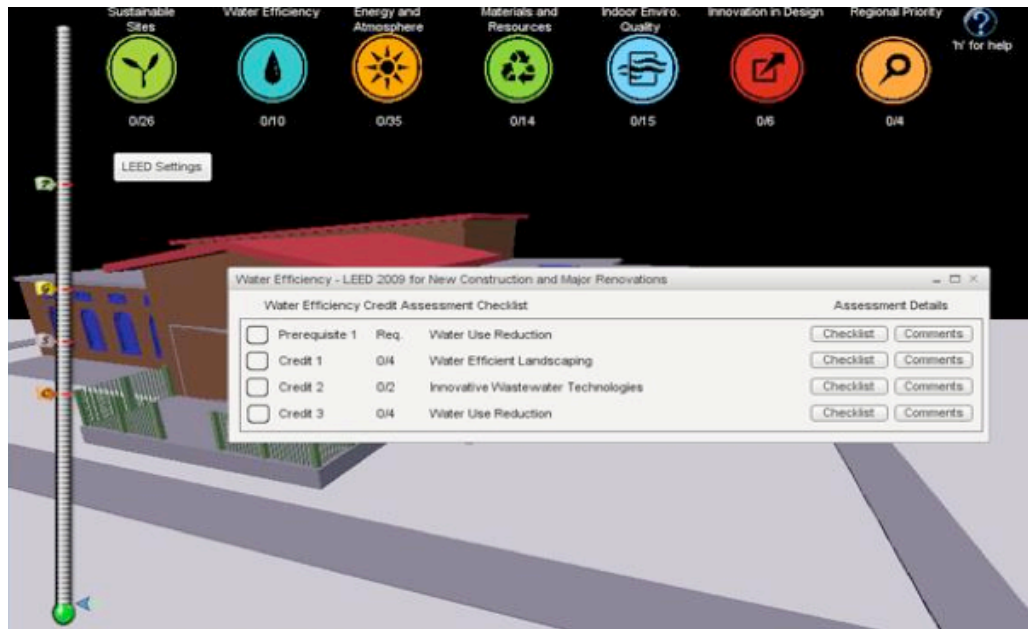
Figure 12. nD BIM Web-Based Software Application Implementing the Developed 6D and nD Framework Utilized in Conjunction with the LEED Energy Standard Portion of the nD Database for LEED Certification Review Analysis of an IFC BIM in a Virtual Environment Linked to the BIMserver.
