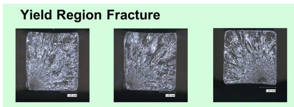
Figure 87. Non-Aged fracture surfaces correlated to the yield region in Figure 86.
