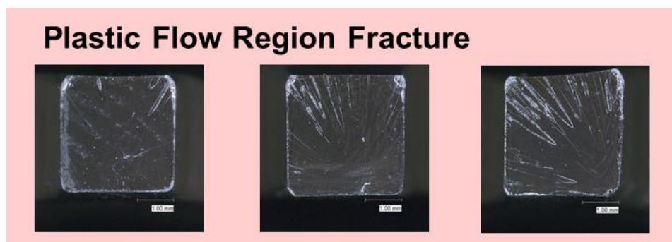
Figure 88. Non-Aged fracture surfaces correlated to the plastic flow region in Figure 86.
