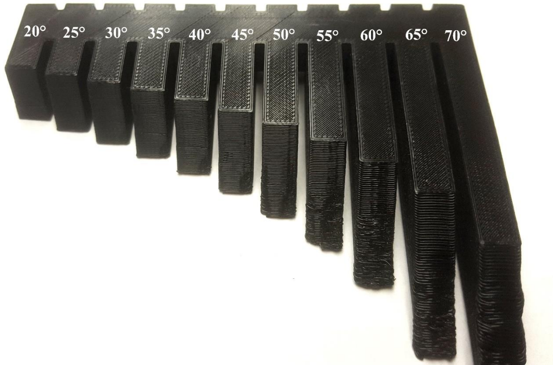
Figure 4.4 Overhang Test Print for Increasingly Steep Angles
