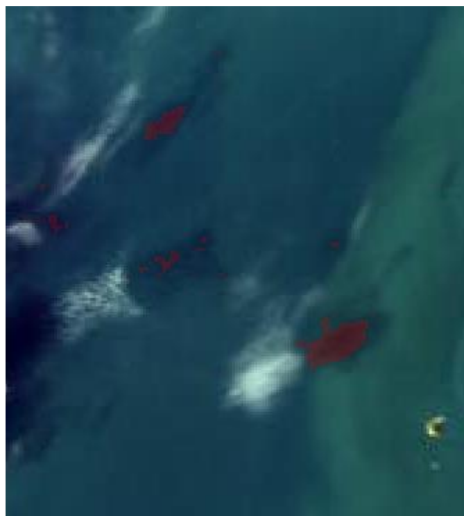
Figure 32. Hong Kong layered image. Shows cloud shadow not detected due to gradient shadow and cloud detection.
