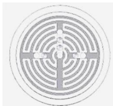
Figure 22. Top Views of the 1" tool mount interdigitated electrode sensor
