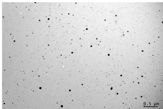
Figure A.2 Lower magnification TEM image of thiol-ene nanoparticles synthesized at 2.5 wt. % organic fraction.
