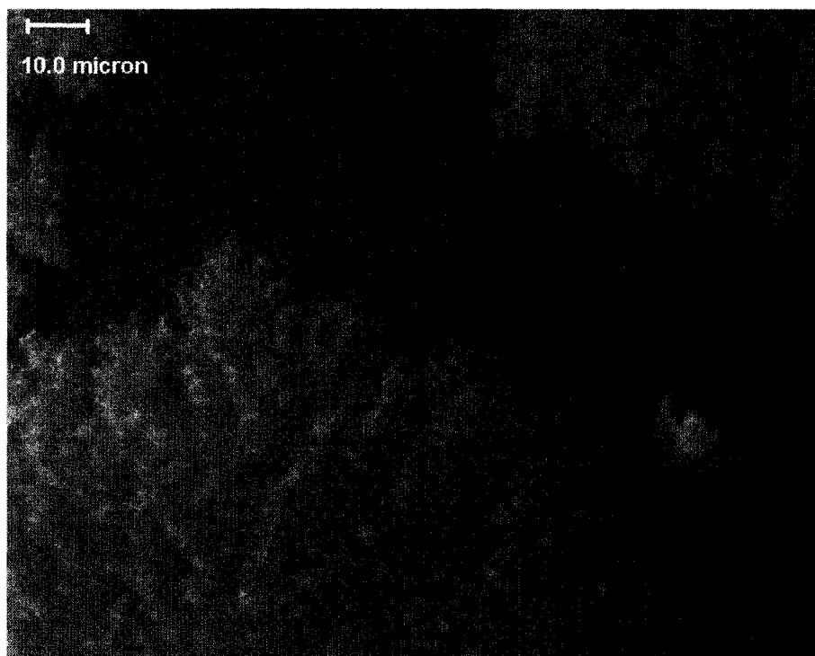
Figure 3.17. Microscope picture of crystallization of the surfactant in the film formed from microemulsion with 15 vol% of diacrylate (HDDA), W = 10 , and 10% water with respect to monomers.
