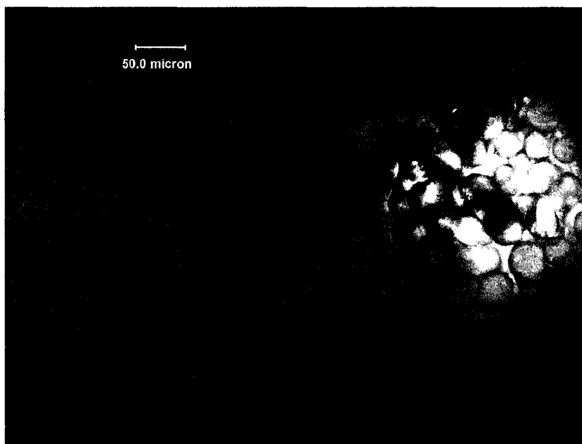
Figure 6.19. Images of a film photopolymerized from a microemulsion based on HDT-APE-DDE with 10 wt% water and W = 10 . (a) Part of a thin film (10 \mu\text{m} ), (b) Top layer of a thick film ( \sim 0.2 mm). The scale bar represents 50 microns.
