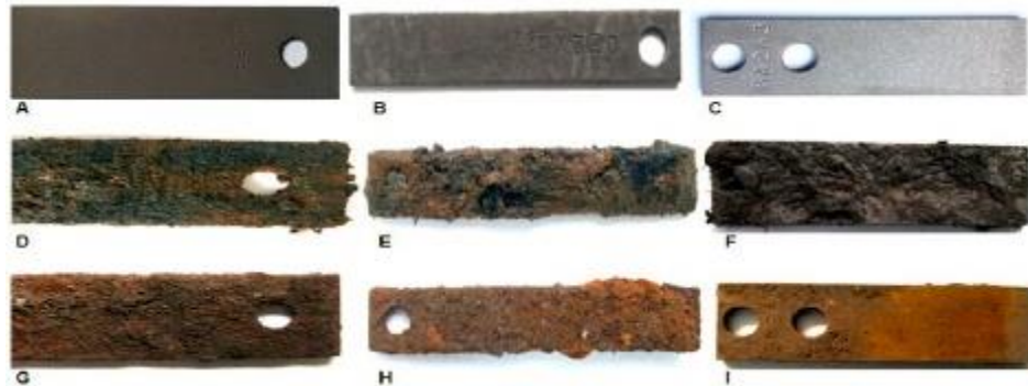
Figure 2. Corrosion of steel specimens. 11
