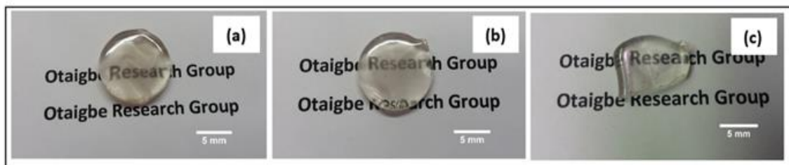
Figure 2.2 Comparison of synthesized Pglass matrix nanocomposites incorporating TSP-POSS prepared by the synthesis method described in the text; (a) neat Pglass, (b) 5 wt.% TSP-POSS, (c) 10 wt.% TSP-POSS.
