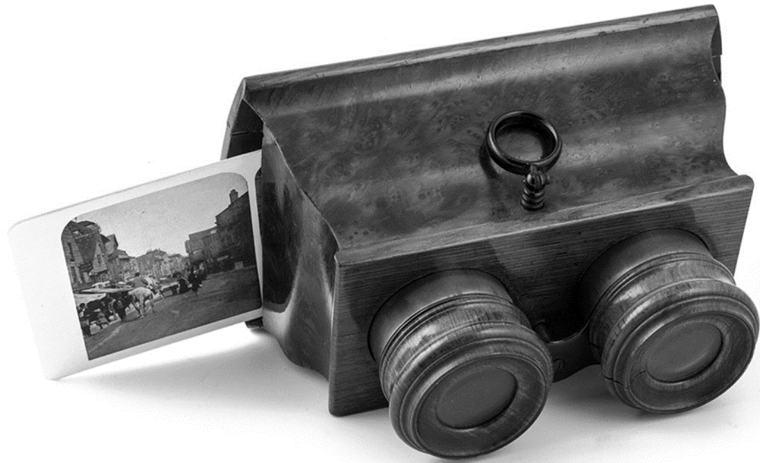
Figure 4. Brewster type stereoscope with stereograph, ca.1848.
