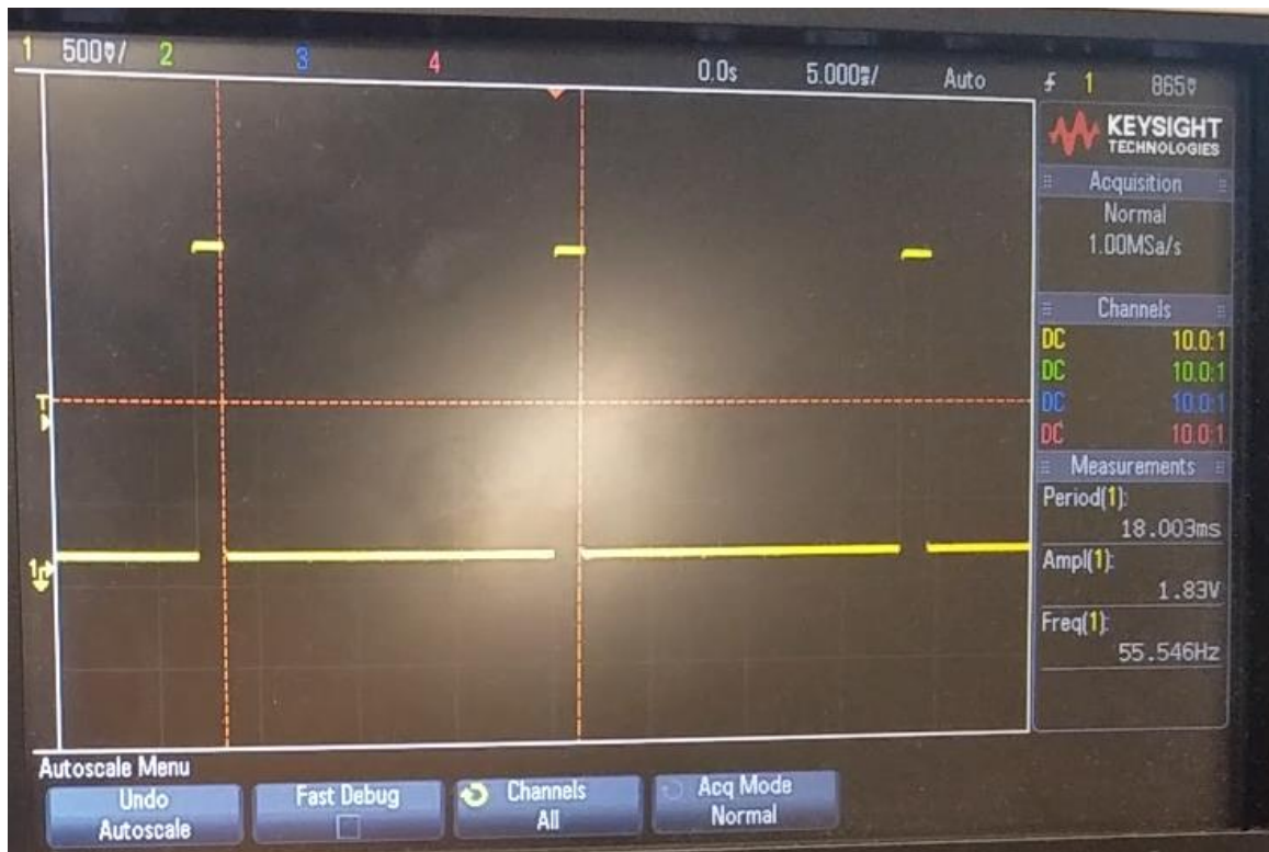
Figure 4.5 Waveform from the Gate to the Flight Controller with the Communication Module Inactive
