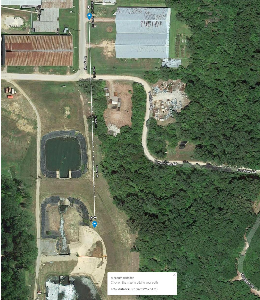
Figure 4.4 RFM69HCW Maximum Distance: 861.26ft
