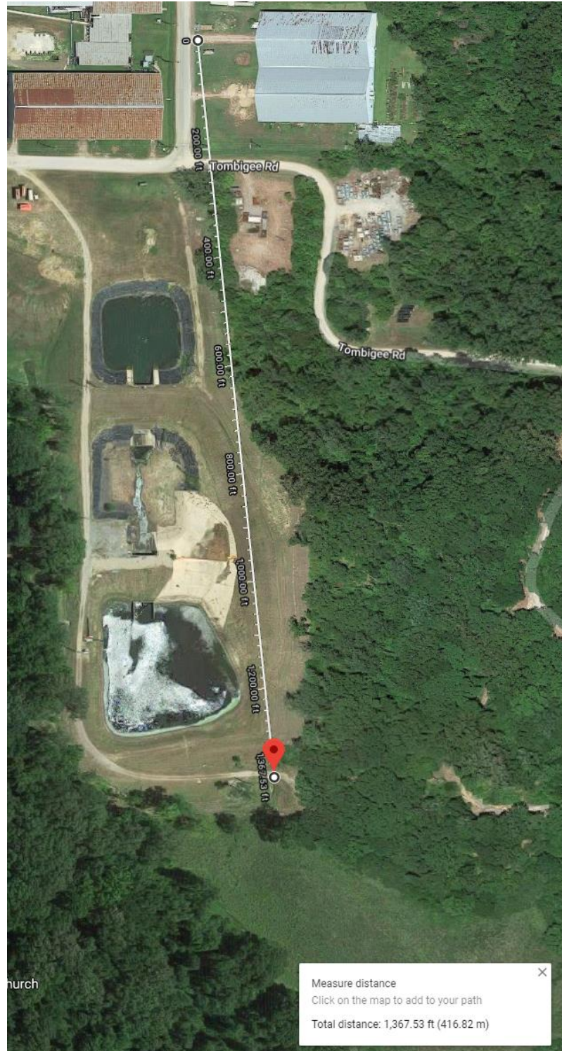
Figure 4.2 LoRa WAN Distance Measurements Maximum Distance: 1,138.79ft
