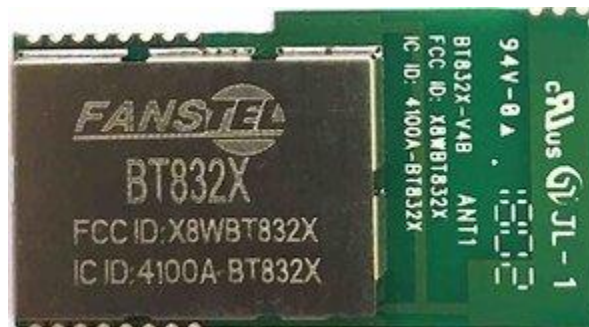
Figure 3.9 BT832X The Longest Range Bluetooth 5 Module [46]
