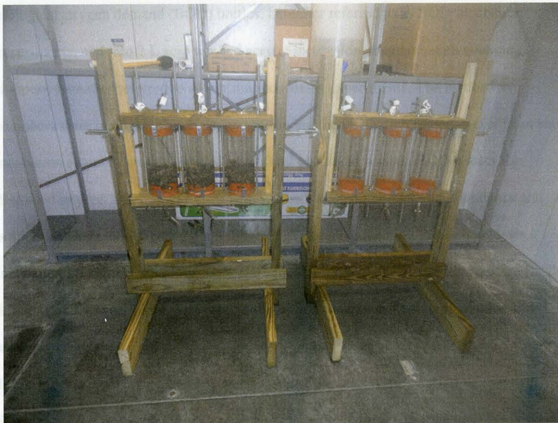
Figure 2. Incubation chamber set-up, with chambers with rubble from the substrage cages pictured on the left and control chambers without rubble on the right.
