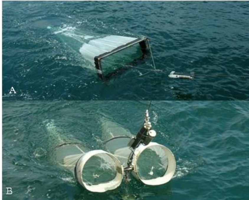
Figure 2. Photographs of the Neuston and Bongo Nets. Top panel (A) shows the Neuston net during a tow, displaying amount of net submerged. Bottom panel (B) shows the bongo nets at the end of a tow.
