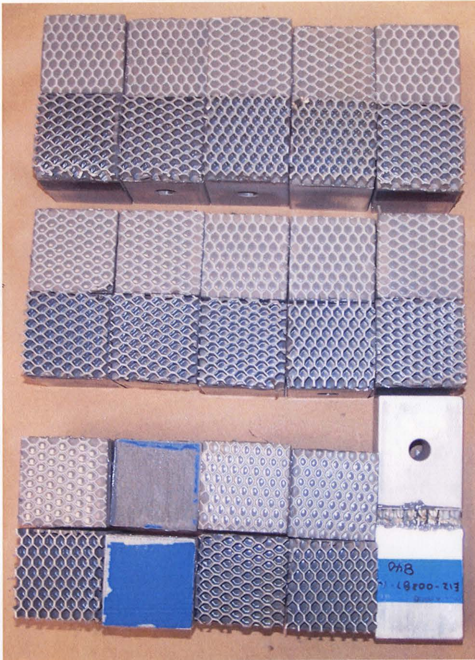
Figure 19. Redux 319 FWT Failed Specimens – RTD Condition. Shown from top to bottom: 90 minute cure cycle specimens, 1x210 minute cure cycle specimens, 4x210 minute cure cycle specimens.
