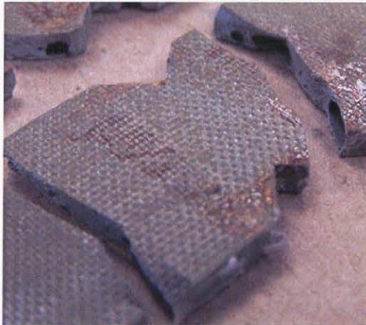
Figure 13. V-notch shear specimen porosity. Many of the V-notch shear specimens exhibited a high degree of porosity along the failure surfaces.
