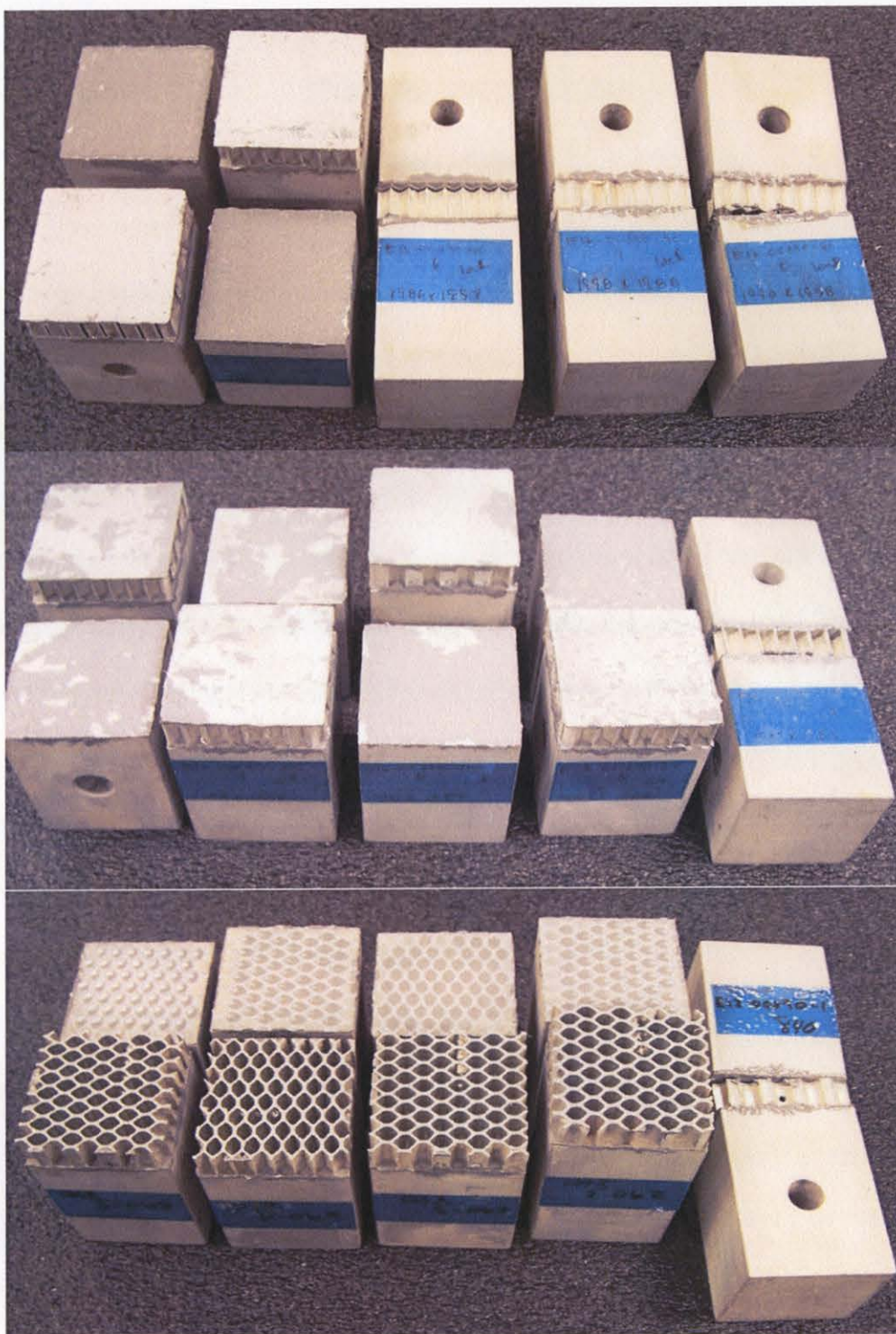
Figure 20. Redux 319 FWT Failed Specimens – 225F Wet Condition. Shown from top to bottom: 90 minute cure cycle specimens, 1x210 minute cure cycle specimens, 4x210 minute cure cycle specimens.
