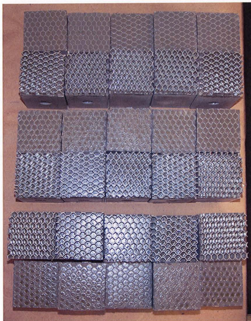
Figure 15. EA9689 FWT Failed Specimens – RTD Condition. Shown from top to bottom: 90 minute cure cycle specimens, 1x210 minute cure cycle specimens, 4x210 minute cure cycle specimens.
