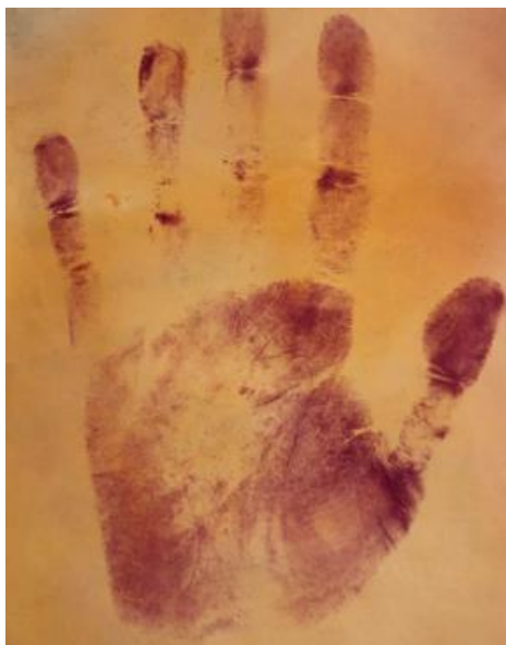
Figure 3: Ninhydrin technique used to develop a print created on white copy paper
