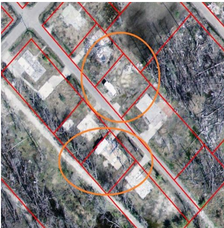
Figure 9: FEMA trailer (FT) shown highlighted in the orange area of interest. FEMA trailers are identified by their length, absence of any structures and are typically on a slab.
